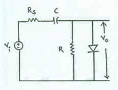
Determine the output voltage waveform for few cycles and indicate its voltage levels.
